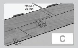
Underlay edges should not be overlapped and butt end edges together. Compressed (Silent) underlay also is useful for cement and concrete floors and ordinary underlay be properly used for other floors as ceramic tiles and stone (Fig. 2).
